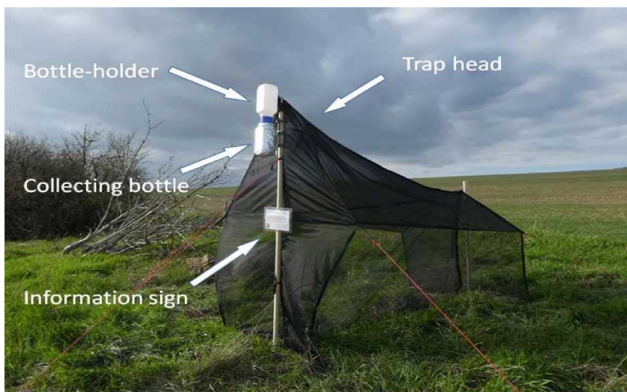
Figure A4.2.1 Malaise trap LTER-Germany type with terms used throughout the protocol
